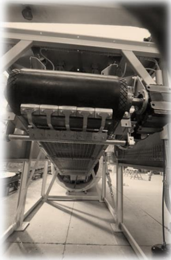
Weighing and inclined belts
